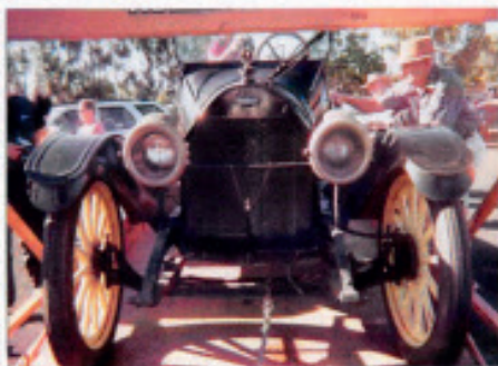
c. 1916 Chevrolet Royal Mail with semi elliptic springs at front and three quarter elliptic springs at rear. The front springs are stiffer (have a higher rate) than the rears to support weight of engine and control steering dynamics of axle. The curved cantilevers at the rear provide insulation from bumps and give a softer ride than would semi elliptics alone, coupled with high ground clearance. (Vehicle courtesy Roger Dunstan, At Dalby, Easter 2009)
