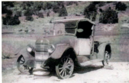
c. 1923 Buick with conventional beam axle/semi elliptic leaf springs. Note snubber plate clamped to front (and rear) of main leaf to increase interleaf friction and provide additional spring damping. (Author's collection)
