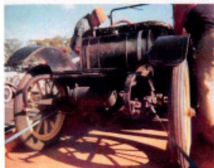
c. 1916 Chevrolet Royal Mail with semi elliptic springs at front and three quarter elliptic springs at rear. The front springs are stiffer (have a higher rate) than the rears to support weight of engine and control steering dynamics of axle. The curved cantilevers at the rear provide insulation from bumps and give a softer ride than would semi elliptics alone, coupled with high ground clearance. (Vehicle courtesy Roger Dunstan, At Dalby, Easter 2009)
